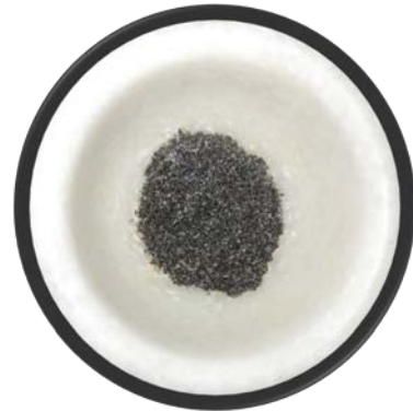
Figure 3 Iron filing and microplastic mixture after segregation
