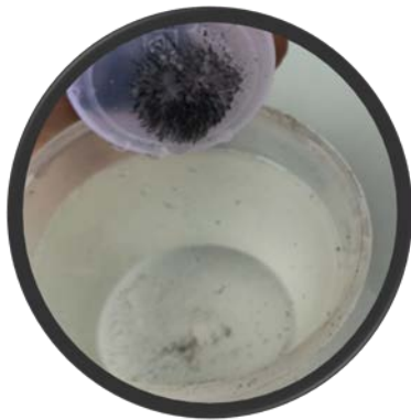
Figure 4 Removal of iron and PET using magnet
